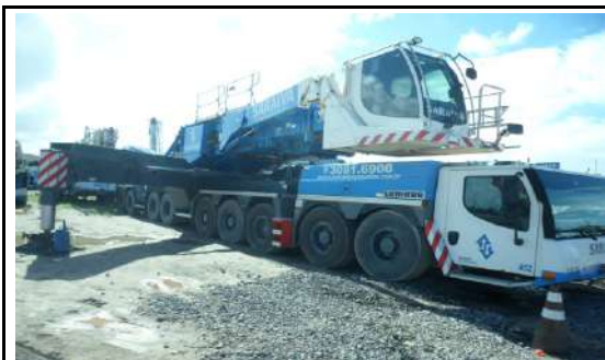
452 - GUINDASTE TELESCOPIO LIEBHERR LTM11200-9.1 2011
